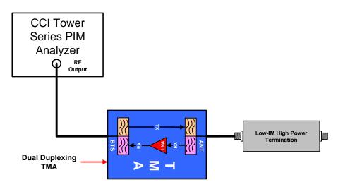
Figure 10 - Dual Duplexing TMA PIM Measurement Test Setup
