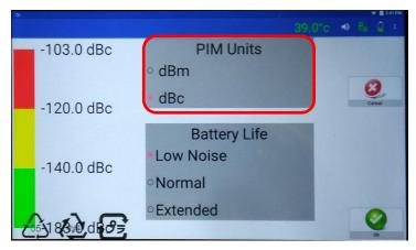
Figure 151 – dBm/dBc Unit Change Selection
