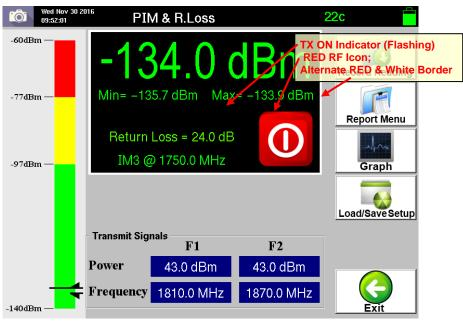
Figure 25 – PIM and Return Loss Window with "TX ON"
