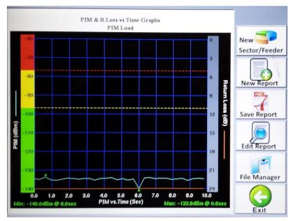
Figure 60 - PIM & Return Loss vs. Time Plot in Report Window
