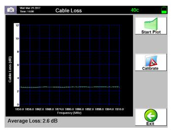
Figure 108 – Cable Loss Measurement
