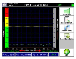
Figure 59 - *PIM & Return Loss vs. Time* Plot (in dBc) on the *PIM vs. Time* Window
