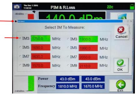
Figure 49 - *IM Select* Window for (IM3) @ Standard F1 = 1810.0 MHz and F2 = 1870.0 MHz
