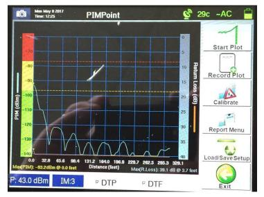
Figure 100 – PIMPoint Measurement of Feed-Line to Antenna
