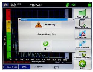
Figure 94 - "Connect Load Std." Warning Pop-up Window
