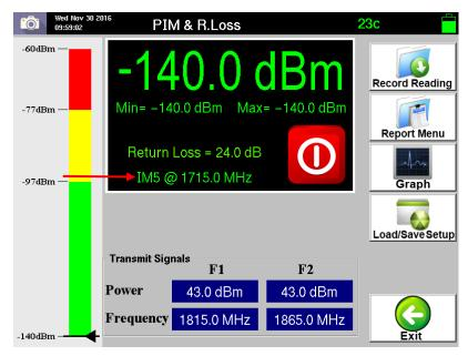
Figure 51 - *PIM and Return Loss* Measurement Window when Set for IM5 Readings
