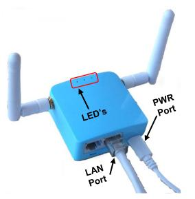
Figure 133 – Wireless Router for Tower Series PiMPro
