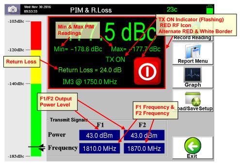
Figure 46 - PIM and Return Loss Window during "TX ON"
