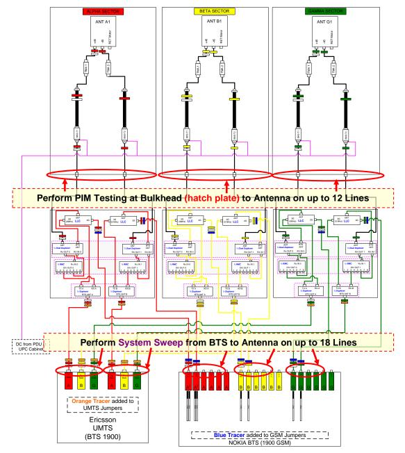
Figure 11 - Required PIM Measurement Points (CCI System Diagram)
