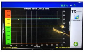
Figure 158 – PIM vs. Time "Graphical" Window
