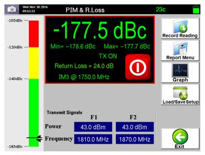
Figure 45 - *PIM and Return Loss* Window during "TX ON" (Reading in dBc)
