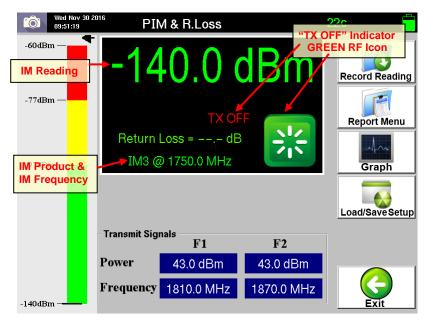
Figure 44 - PIM and Return Loss Window during "TX OFF" (Reading in dBm)
