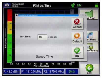
Figure 53 - Configure PIM vs. Time Parameters Window
