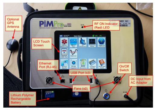
Figure 12 - Overall view of the CCI Tower Series PIM Analyzer
