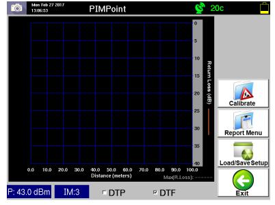
Figure 80 – Distance to Fault (DTF) Selected
