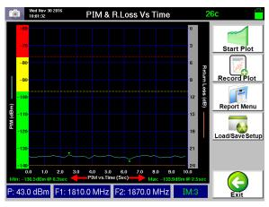
Figure 58 - PIM & Return Loss vs. Time Plot on the PIM vs. Time Window
