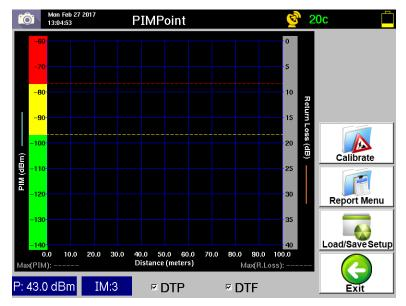
Figure 81 – Distance to PIM and Distance to Fault (DTP & DTF) Selected
