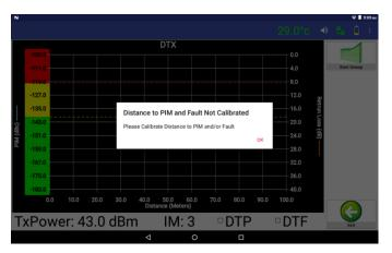
Figure 160 – PIMPoint Not Available Screen Due to No Calibration Performed
