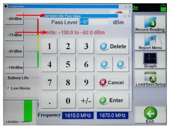
Figure 43 - "Set Meter Min Pass Value" Window
