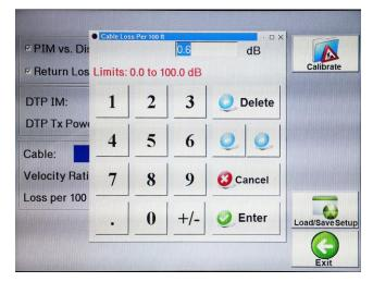
Figure 88 - Cable Loss per 100 ft pop-up window
