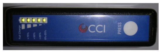
Figure 168 – Fully Charged Battery LED Status Indicators
