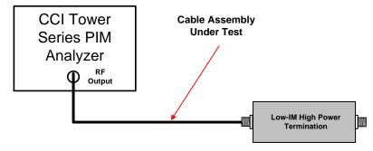
Figure 4 - Cable Assembly PIM Measurement Test Setup
