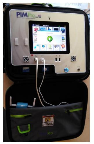
Figure 132 – Wireless Router Mounted in PiMPro Carrying Case
