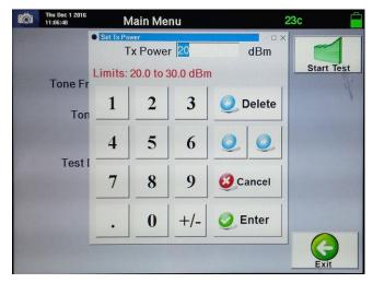
Figure 74 – Set Tx Power for DAS Tx Generator
