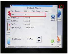
Figure 165 – Battery Status (1%) after Pressing Battery Icon
