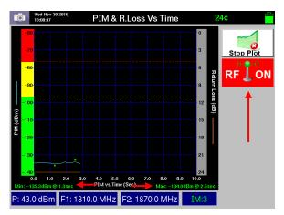
Figure 57 - Partial *PIM & Return Loss vs. Time* Plot on the *PIM vs. Time* Window Showing *Stop Plot* and *RF ON*
