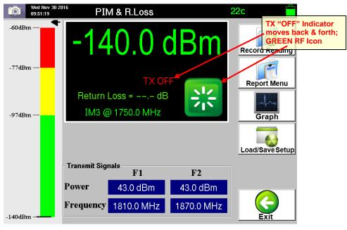
Figure 24 - PIM and Return Loss Window with "TX OFF"
