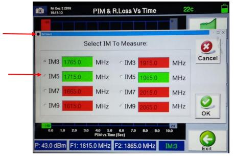
Figure 50 - *IM Select* Window for IM5 at F1 = 1815.0 MHz and F2 = 1865.0 MHz
