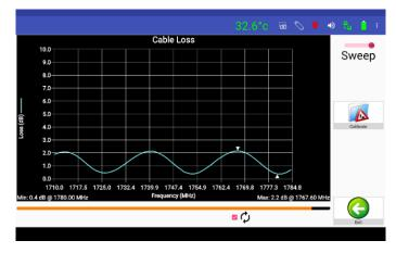
Figure 45 - Cable Loss Measurement
