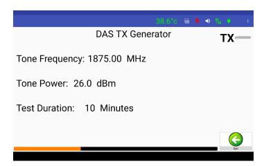
Figure 29 – DAS TX Generator Test Window
