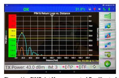
Figure 41 – PIMPoint Measurement of Feedline to Antenna
