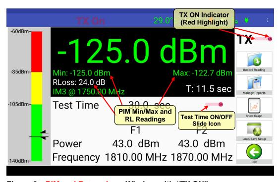
Figure 9 - PIM and Return Loss Window with "TX ON"
