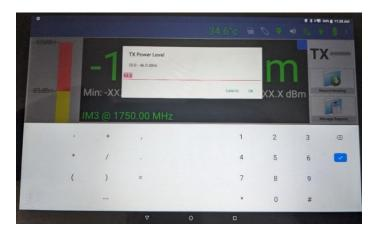
Figure 20 - Set Tx Power Per Channel Window
