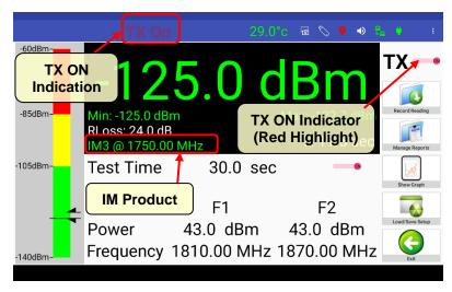
Figure 23 - PIM and Return Loss Window during "TX ON"
