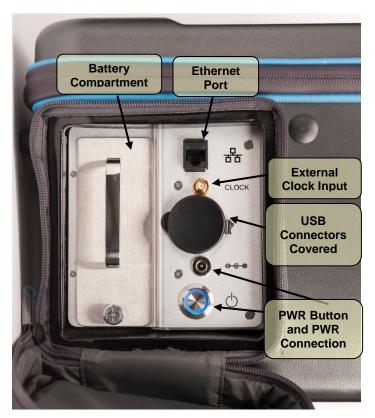
Figure 3 - Power, Ethernet, Battery, USB and Other Connections Access
