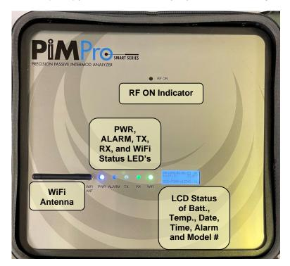
Figure 1 - View of the CCI PiMPro Smart Series PIM Analyzer Main Panel
