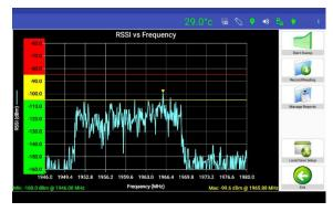
Figure 25 - Completed RX Interference Sweep Window
