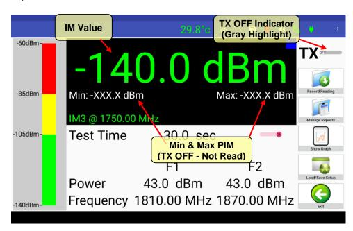
Figure 8 - PIM and Return Loss Window with "TX OFF"
