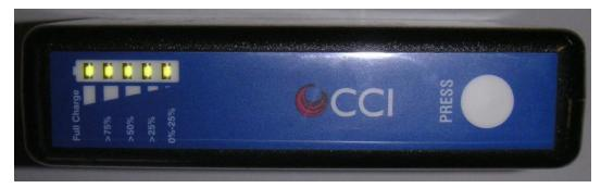
Figure 69 - Fully Charged Battery LED Status Indicators
