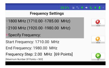
Figure 24 - Configure Frequency Parameters Pop-up Window
