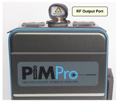
Figure 2 - PiMPro Smart Series RF Output Port
