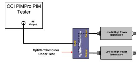
Figure 8 - Splitter/Combiner PIM Measurement Test Setup
