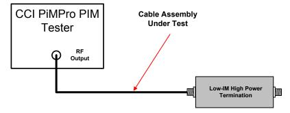
Figure 4 - Cable Assembly PIM Measurement Test Setup
