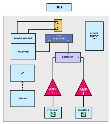
Figure 2 - PiMPro Block Diagram
