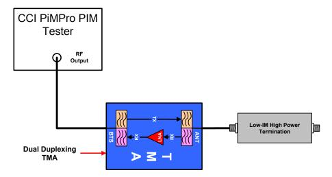
Figure 10 - Dual Duplexing TMA PIM Measurement Test Setup
