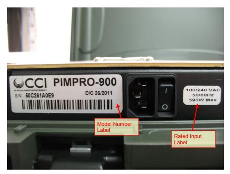
Figure 13 - Model Number and Rated Input Label Location
