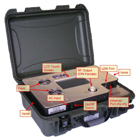
Figure 12 - Overall view of the CCI PiMPro PIM Analyzer
