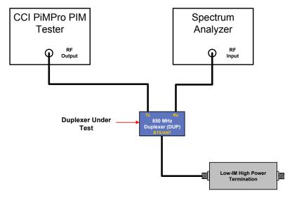
Figure 6 - Duplexer PIM Measurement Test Setup
