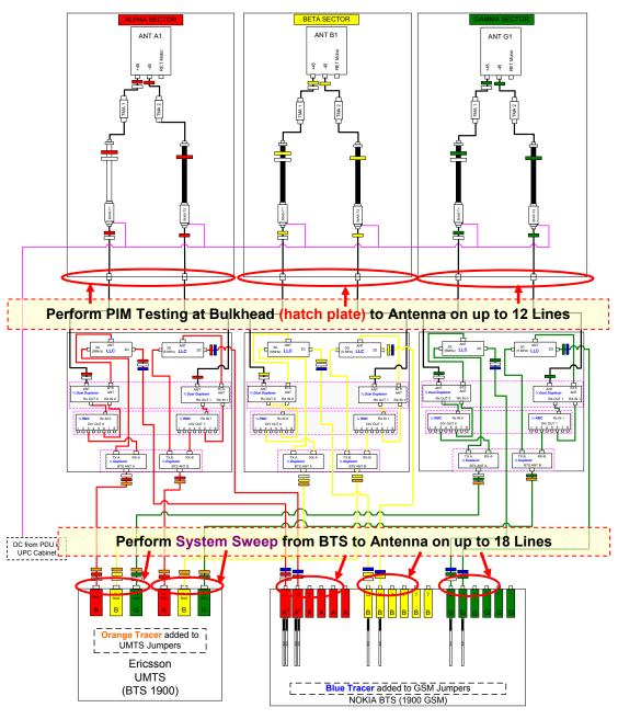
Figure 11 - Required PIM Measurement Points (CCI System Diagram)
