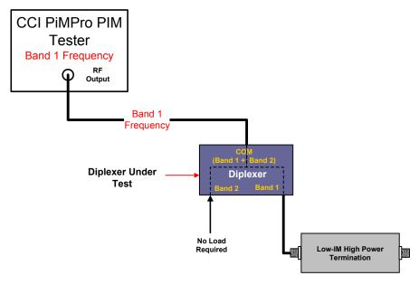
Figure 7 - Diplexer PIM Measurement Test Setup
