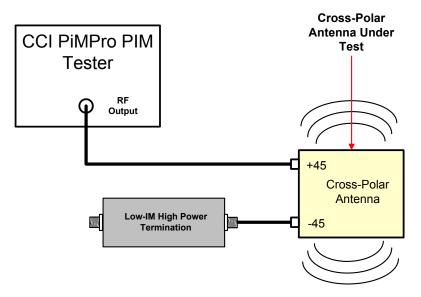
Figure 5 - Cross-Polar Antenna PIM Measurement Test Setup
