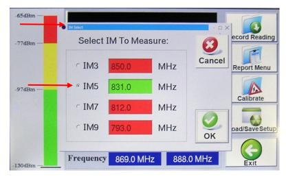
Figure 45 - *IM* Select Window for IM5 at F1 = 869.0 MHz and F2 = 888.0 MHz
