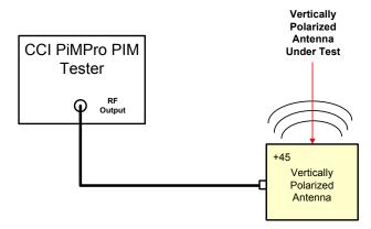
Figure 3 - Vertically Polarized or Omni-directional Antenna PIM Measurement Test Setup
