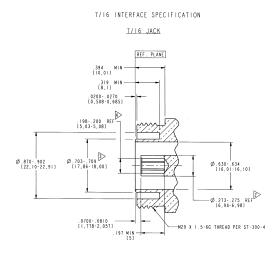
Figure 16 - DIN-Female Interface Drawing
