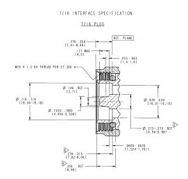
Figure 15 - DIN-Male Interface Drawing
