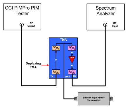
Figure 9 - Duplexing TMA PIM Measurement Test Setup
