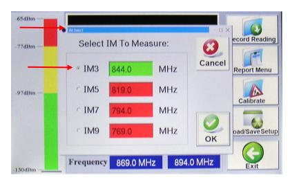
Figure 44 - IM Select Window for (IM3) @ Standard F1 = 869.0 MHz and F2 = 894.0 MHz
