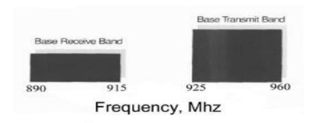
Figure 1 - GSM Band Plan
