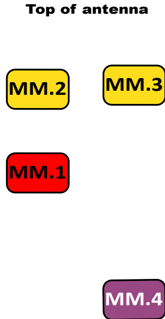
RET placement as viewed from rear of antenna
