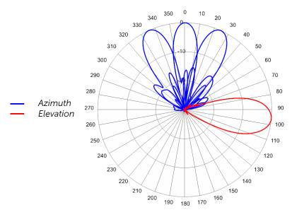
915 MHz Azimuth with Elevation 6°
