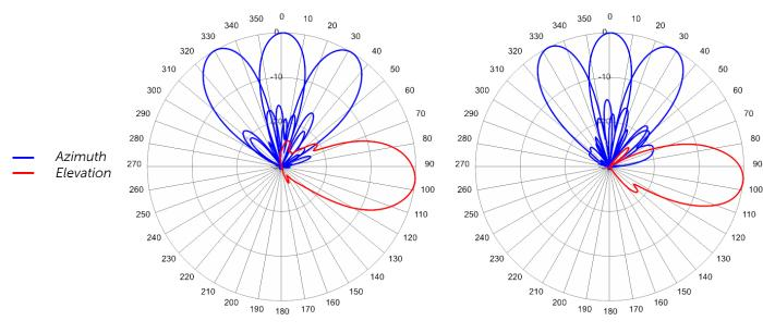
740 MHz Azimuth with Elevation 6°
