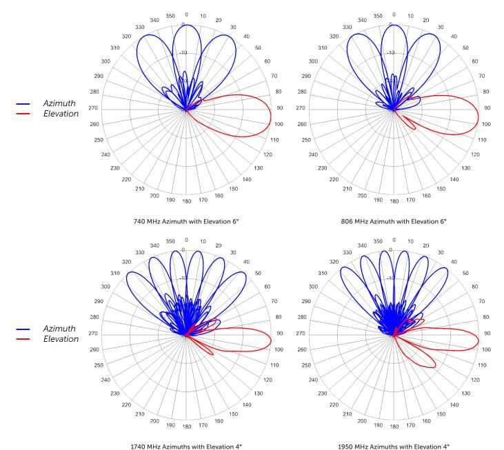
1950 MHz Azimuths with Elevation 4°
