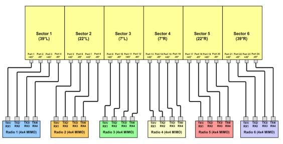
MBM Series "U Band" Multisector Antenna (4x4 Connection)
