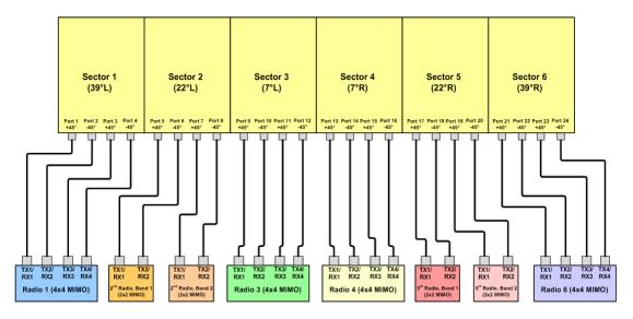
MBM Series "U Band" Multisector Antenna (4x4\_and\_2x2 Mixed Connection)
