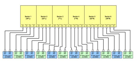
MBM Series "U Band" Multisector Antenna (2x2\_Two Band Connection)
