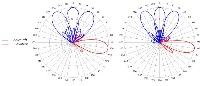
734 MHz Azimuth with Elevation 10°
