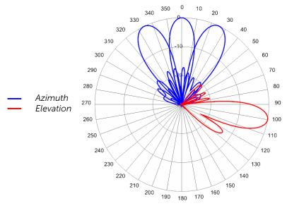
880 MHz Azimuth with Elevation 10°
