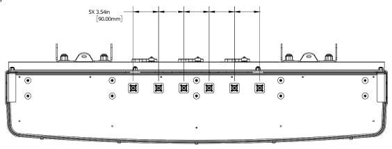
RET to Element Configuration MBA3R-B3AA and MBA3R-B3AB Element and RET configuration (Type 1 External RET)
