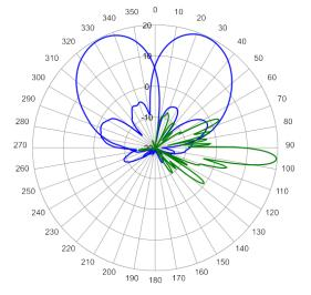
2350 MHz Azimuth Elevation 5°
