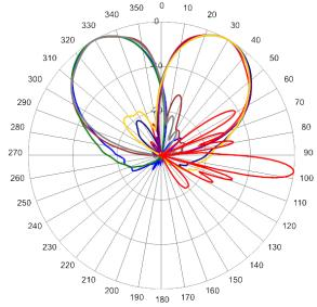
1780 MHz Azimuth with Elevation 7°
