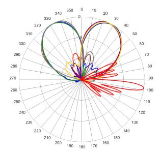
2180 MHz Azimuth with Elevation 7°
