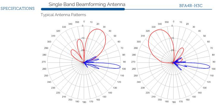
3500 MHz Azimuth 30° with Elevation 7° Service Beam
