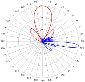
3500 MHz Azimuth with Elevation 7° Broadcast Beam
