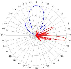
3920 MHz Azimuth 0° with Elevation 7° Service Beam
