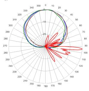
2360 MHz Azimuth with Elevation 4°
