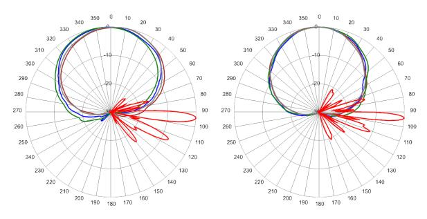
1720 MHz Azimuth with Elevation 4°
