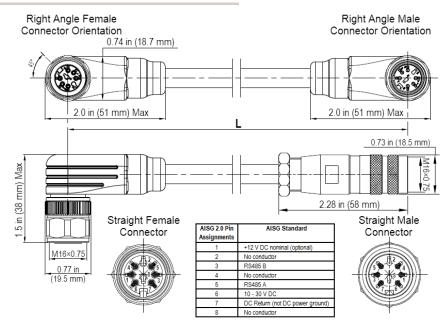
AISG-Male to AISG-Female Jumper Cable
