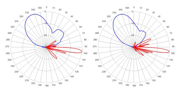
3500 MHz Azimuth with Elevation 7° Soft Split
