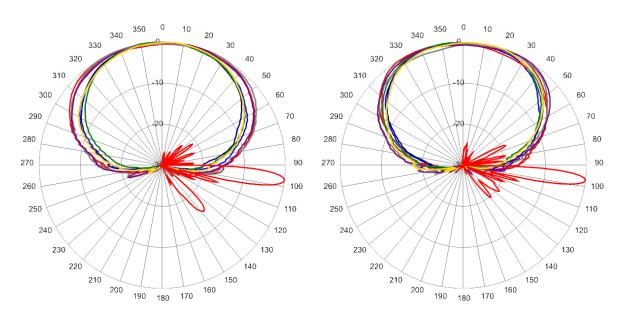
3500 MHz Azimuth with Elevation 7° Single Column
