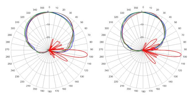
734 MHz Azimuth with Elevation 7°
