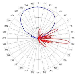
3500 MHz Azimuth with Elevation 7° Broadcast Beam
